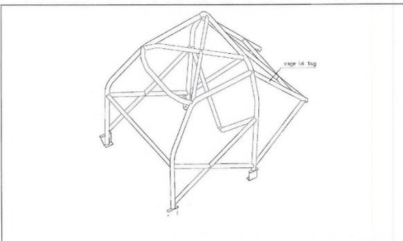
This Roll Over Protection System has been designed to meet current FIA Appendix J regulations, in particular Appendix J, articles 253.8.2 and 253.8.3.
