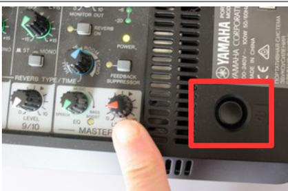
A close-up photograph of the Yamaha control panel. A finger is shown pressing a power button. A red square highlights the power button. A green LED indicator light is visible above the power button.               |
